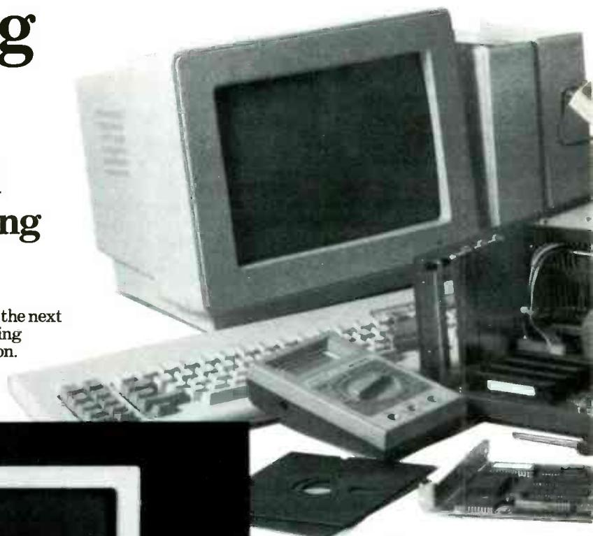
You assemble and test your computer's "intelligent" keyboard, install the power supply and 5 1/4" disk drive, then interface the high-resolution monitor. But that's not all.
