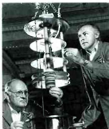
**WESTINGHOUSE TECHNICIANS** Don Martin and Ray Malingowski make connections for a test run of the complete assembly of the electrical lead that set a world record for current carried by a practical, high-temperature superconductor.
