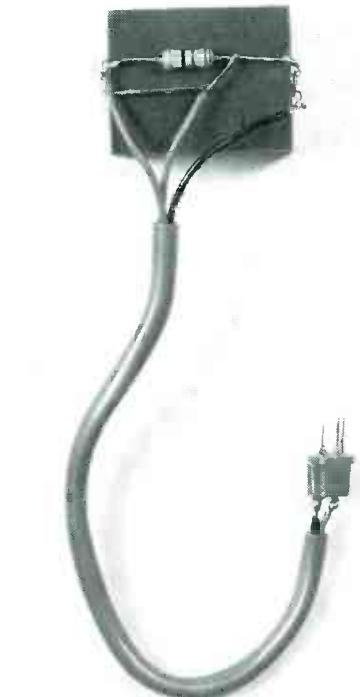
**PROTOTYPE VERSION** of the simulated laser diode. A hole drilled in the block provides a light path.
