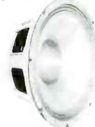
12" woofer made in the USA by Eminence. Paper cone and dust cap with treated cloth surround. 80 oz. magnet. 2-1/2" vented voice coil. 8 ohm. 170W RMS, 255W max 40-4.5KHz response.
